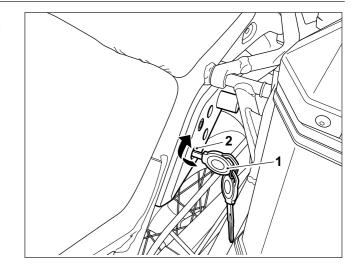
**2** Lift the front of the passenger seat (1) clear of the rider seat (2) and slide the passenger seat towards the front of the motorcycle to remove, as shown. Retain the passenger seat for reuse.
