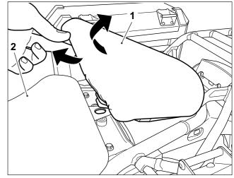
**21** Fit the touring passenger seat to the motorcycle ensuring the retainer (1) on the rear of the seat locates correctly in the motorcycle frame (2).
