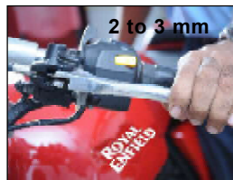
Clutch Lever (free play 2 - 3 mm)
