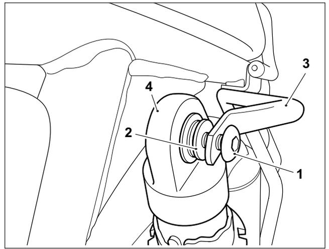
**2** Remove the front grab rail fixing (1) securing the lift handle (2) to the motorcycle frame (3). Remove the lift handle from the motorcycle.
