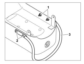
**2** Remove the seat rear fixings (1) and nuts (2) from the left hand and right hand side of the motorcycle. Remove the seat.
