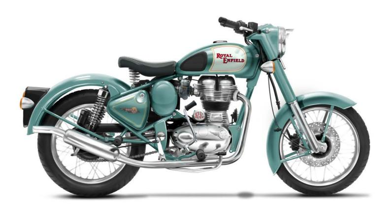
Royal Enfield handled the challenge by dividing the design task into two parts. In the first part, all the electronic and modern components were positioned on the vehicle layout in such a way that they were least exposed, and wherever they were exposed, they were placed in such a way that they blended with the aesthetic lines of the motorcycle without disturbing the visual harmony of the design.
